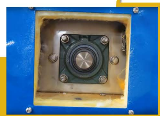
Easy External Access to High-Temperature Bearings
