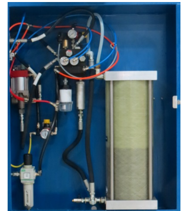
Manifold Block Hydraulics (Inside Cabinet)
