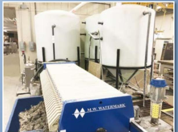
**Capital Granite is using an M.W. Watermark filter press to help recycle the process/waste water that is used throughout their fabrication shop.**
