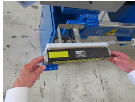
The Safety Buttons on Each Side Are Recessed to Help Prevent Operator Override
