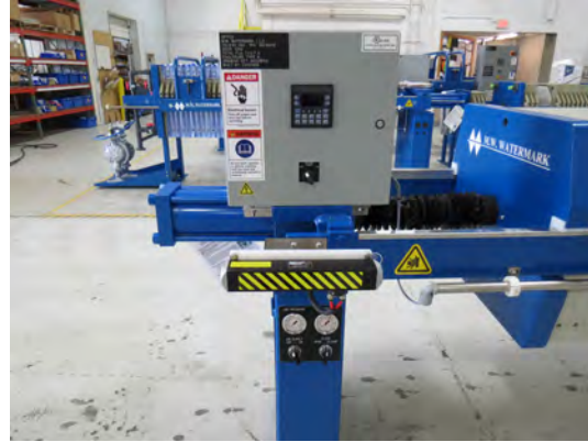
M.W. Watermark 630mm Filter Press with Optional Two-Hand Hydraulic Safety Interlock
