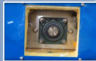
Easy External Access to High-Temperature Bearings
