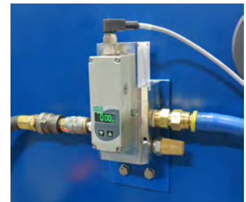
AFPCS Pump Control Mounted to Filter Press
